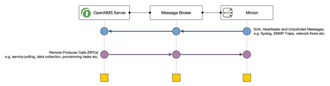
This section describes how you can setup *OpenNMS Horizon* to use other supported messaging systems for the communication with *Minions*.
