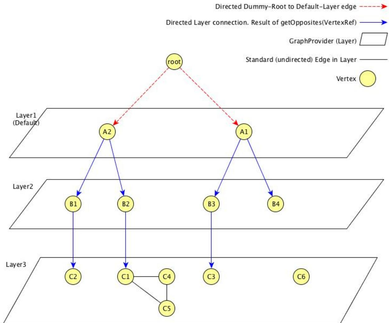
From the given example, the user can select the **Breadcrumb Example** Topology Provider from the menu. The user can switch between **Layer 1**, **Layer 2** and **Layer 3**. In addition for each vertex which has connections to another layer, the user can select the **navigate to** option from the context menu of that vertex to navigate to the according layer. The user can also search for all vertices and add it to focus.
